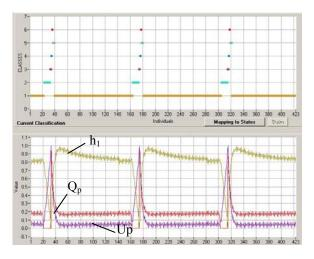
Figure 7. a : Training data: failure scenario: pump blockages b: Classification results.
